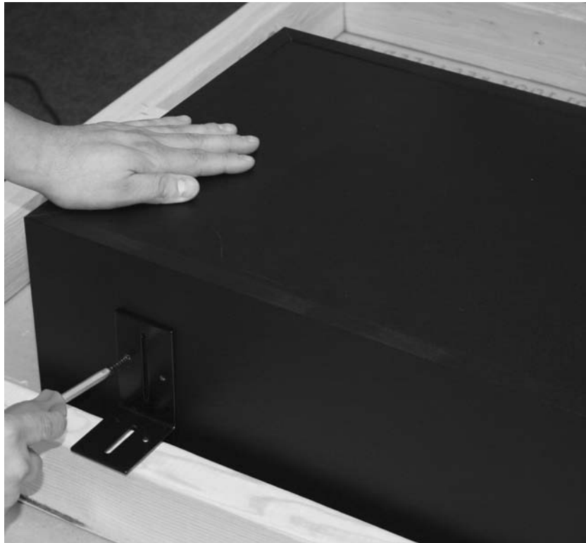
Figure 2: Mount brackets on subwoofer cabinet.
